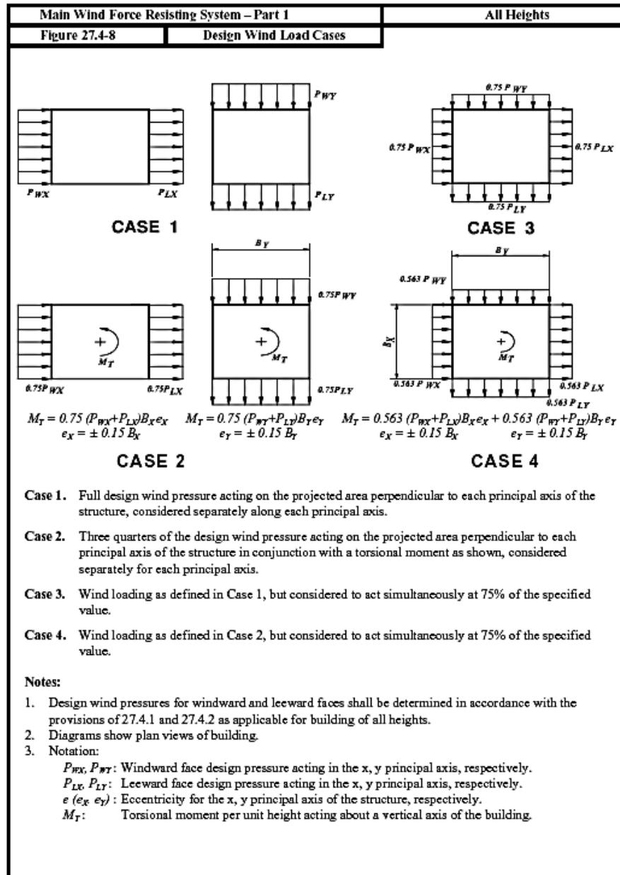
Figure 27 Design wind load cases from ASCE 7-10
