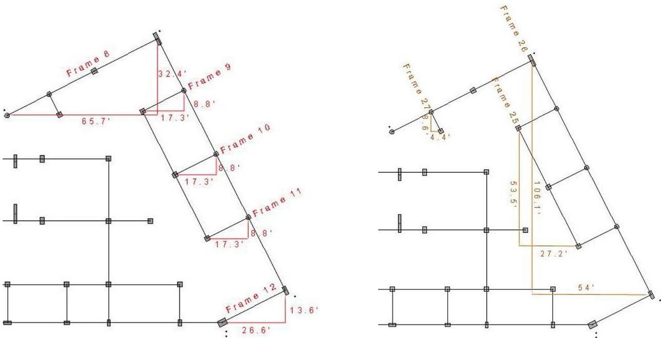
**Figure 29** Frames 8-12 (left) and frame 25-27 (right) separated into their corresponding X-and Y-components
