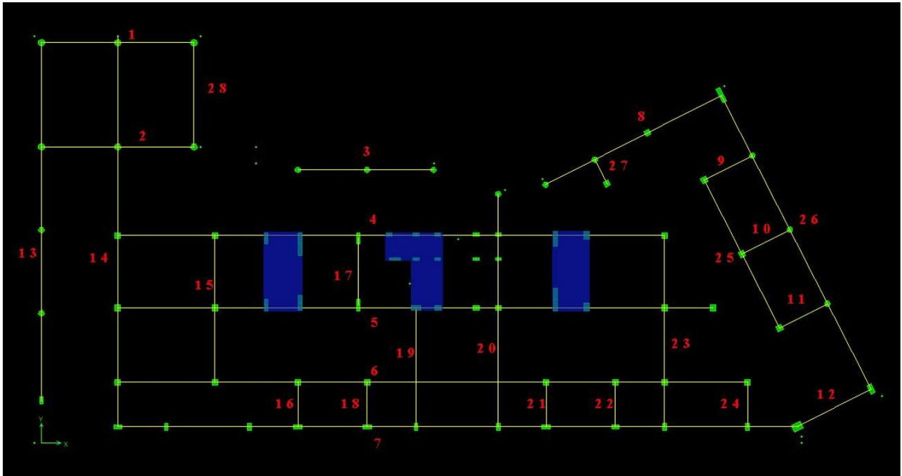
**Figure 25** Moment frame layout with frame assignments
