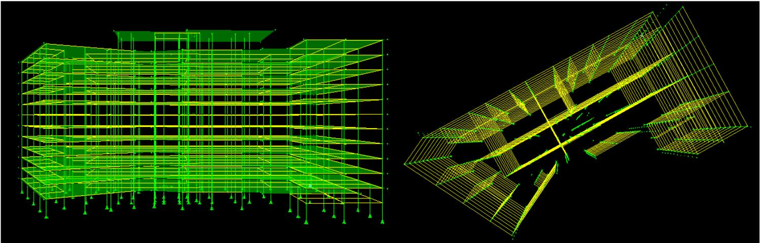
**Figure 24** 3D perspectives of equivalent frames with rigid diaphragm (left) and bird's eye view of the moment frames (right) where the vertical green lines are the columns and horizontal yellow lines are the beams
