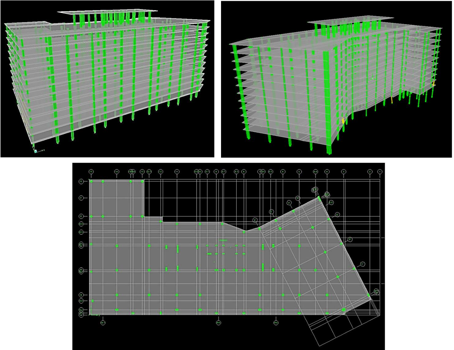
**Figure 22** 3D perspectives (top) and plan view (bottom) of the existing lateral system modeled in ETABS
