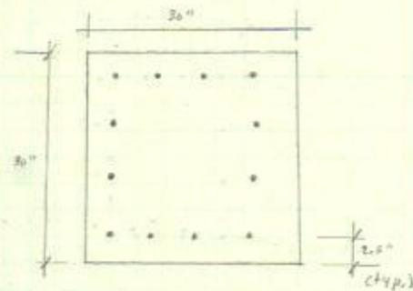
assumption: column is subjected to only gravity load  $\therefore$  check the column for pure axial compressive strength
