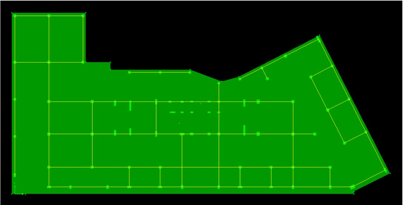
**Figure 23** Plan view of the rigid floor diaphragm (green) and moment frame locations (yellow lines)
