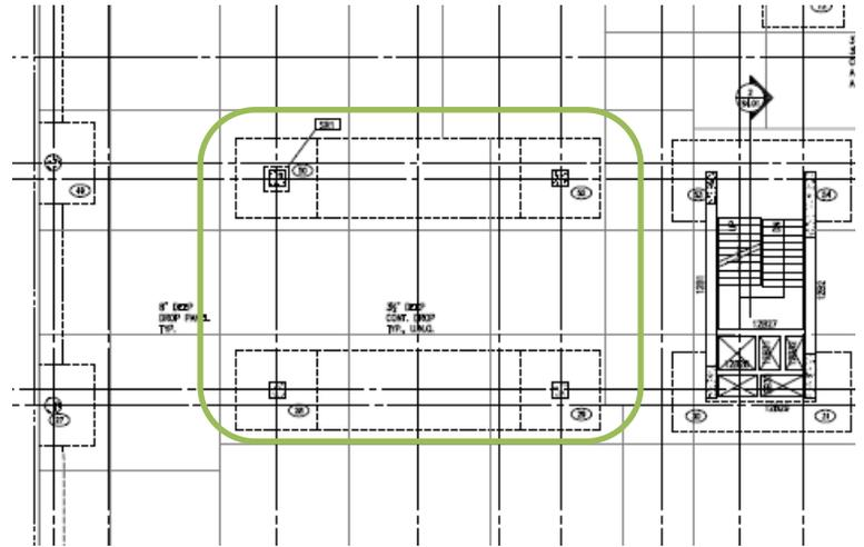
Figure 15 Interior flat slab panel
