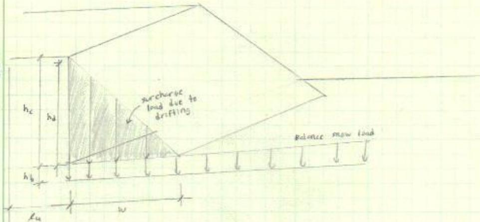
step 6: maximum intensity of the drift surcharge load,  $p_d \rightarrow$  Sect 7.7.1
