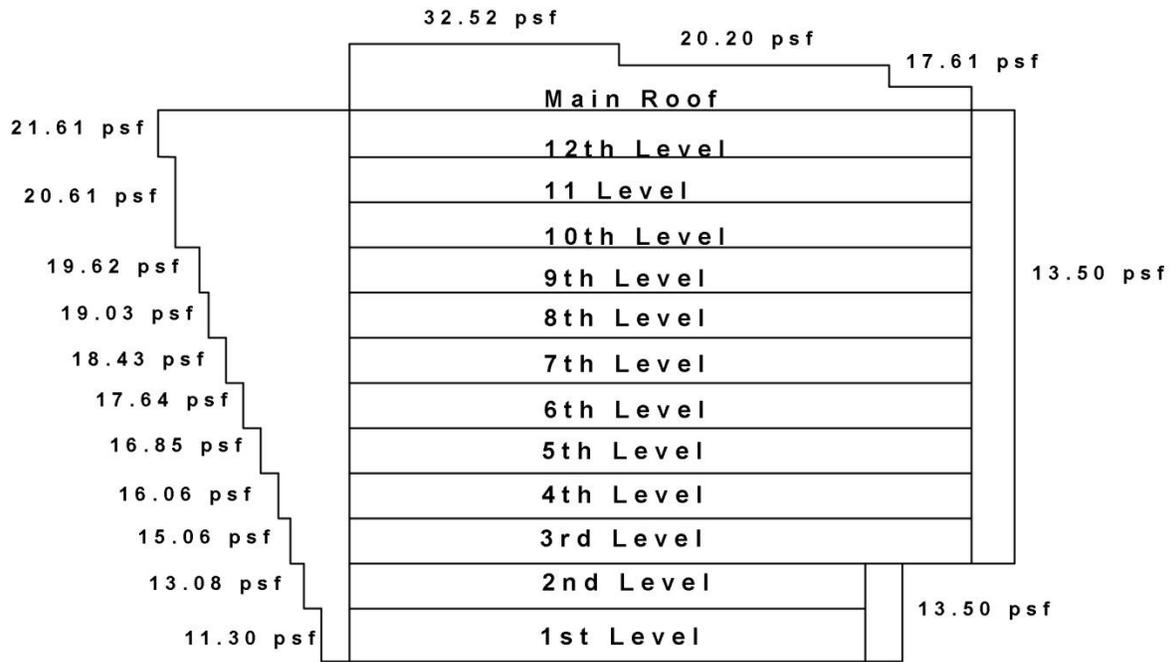
**Figure 18** N-S wind pressure vertical pressure sketch
