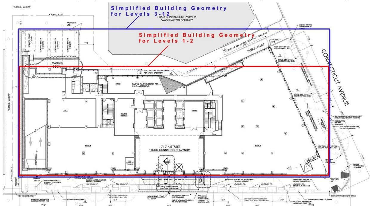
**Figure 17** Simplified building shape for wind load analysis
