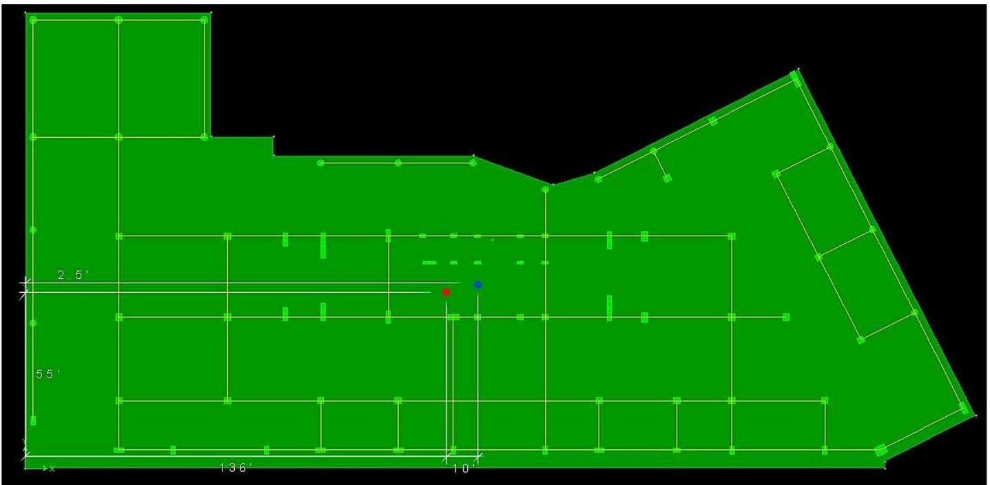
**Figure 28** Plan view showing the location of the Center of Mass (blue dot) and the Center of Rigidity (red dot)
